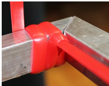
Single sided weaving requires that the direction of the wrap change so the weave stays on the top side. Wrapping the plastic around the cross strand changes its direction.
